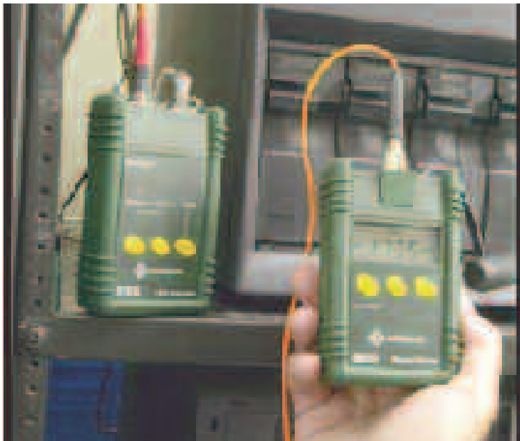
MTCK-002 Single-mode Test Kit.
